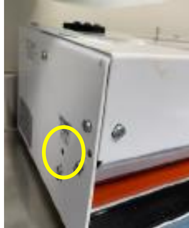
Teflon rotating knob missing
